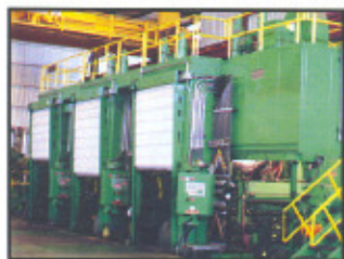
BUSCH mill window closures under test following fabrication.
